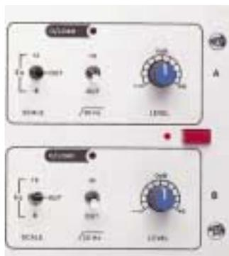
In order to offer operational flexibility a variable fader resolution has been incorporated i.e. 6 or 12 dB cut or boost. This function ("scale") is combined with the bypass switch, which silently removes the graphic equaliser section from the signal path. A subsonic 18dB/octave roll off filter (-3dB @ 3Hz) can be switched in or out from each of the channels.
